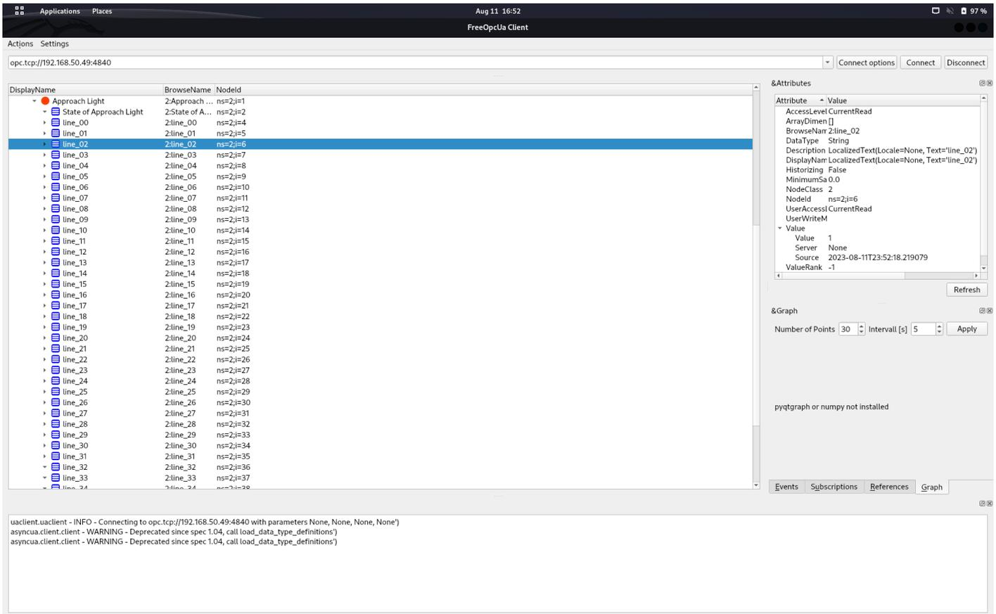
We can see `line_xx` objects, where `xx` is a two-digit number from 0 to 34 (35 in total). Each value is either a 1 or a 0 and changes approximately once a second. There is also a `ts` object, which dumps a timestamp in the ISO 8601 format. `State of Approach Light` turned out to be a red herring.
