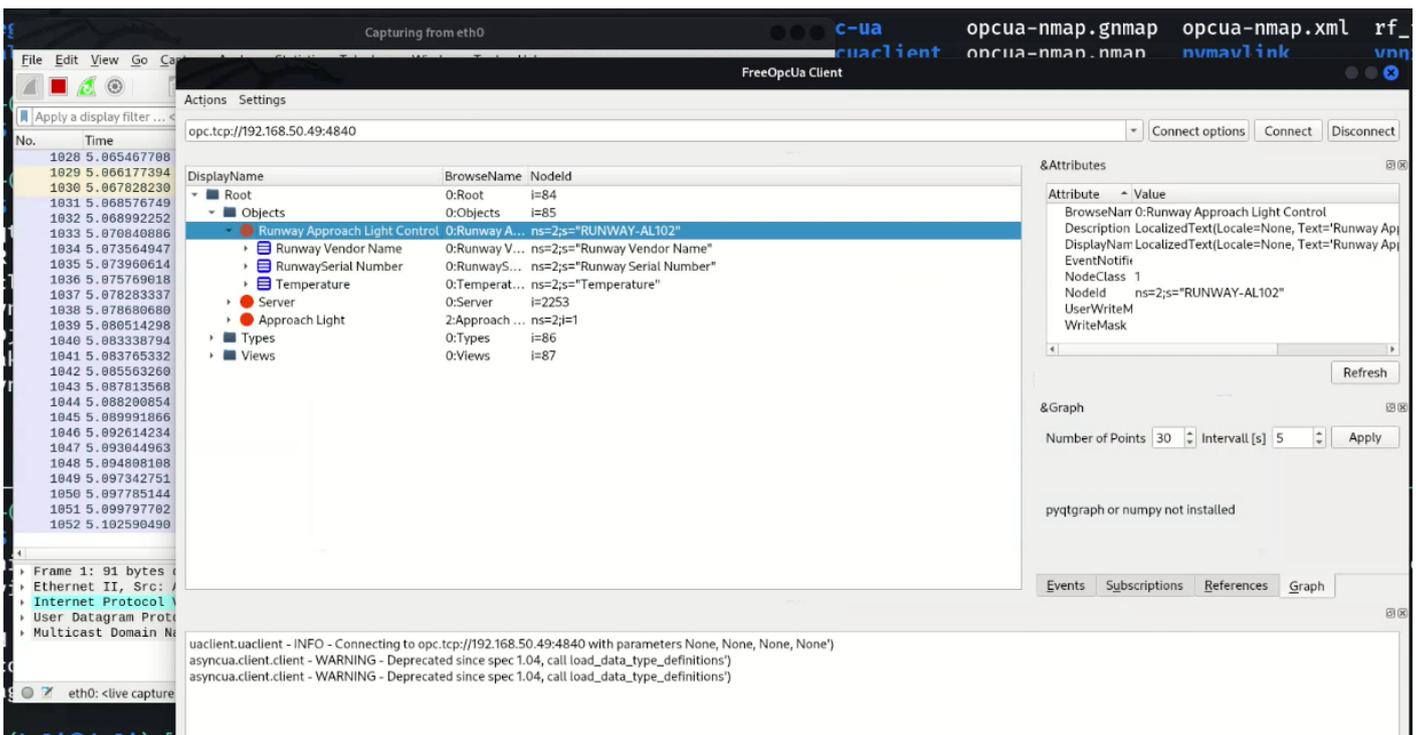
This screen shows us a few things. First, anonymous, unauthenticated sign in is allowed. Second, two custom objects exist: `Runway Approach Light Control` and `Approach Light`. The `Server` object is standard in PLCs that use the OPC UA protocol.
